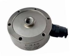
The FC-2300A pan cake type load cell is available in metric capacities. It has largest capacities of our load cell 500 kg to 75 ton in metric thread. Most of capacities feature  $\sim 2mV/V$  output built in to alloy steel design.
